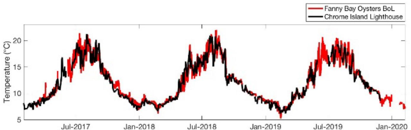
Figure 1. Daily measurements of surface seawater temperature made at Chrome Island Lighthouse compared to five minute averaged temperatures from the Burke-o-Lator (BoL) installed at Fanny Bay Oysters in Baynes Sound, BC.
